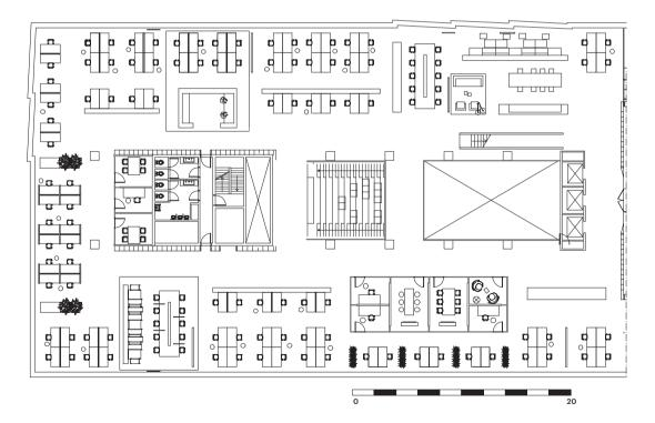
The office floors measure 33 by 82 metres, what is unusually large by Dutch standards. To bring daylight into these spaces, the architects created a large atrium in the middle and several small ones along the facade. Open staircases have been used to connect the floors.
