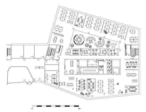
The building has compact office floors (approx. 80 workstations per floor unit). Workspaces are located around a central core which houses a kitchenette, toilets and storage. A central atrium ensures that all spaces have access to daylight.
