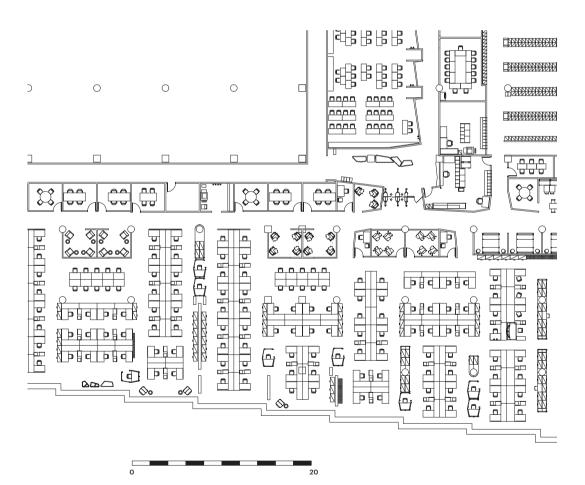
The building has a deep floor plan, which makes it difficult to provide daylight and outside views in all work settings. To deal with this, all open workstations are located along the facade, while facilities for temporary use (i.e. meeting rooms, kitchenette, informal areas) are located towards the centre of the floor.
