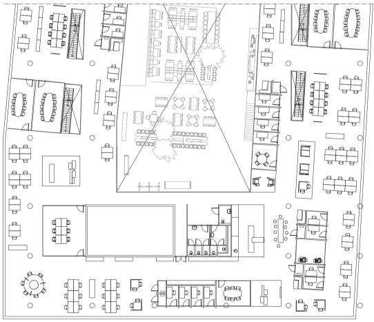
By Dutch standards, the office floors are unusually large. The enclosed spaces (meeting rooms, focus rooms) are positioned so as to break up the large floor plates into smaller areas. The stairs in the atrium were added to improve connections between the different floors.
