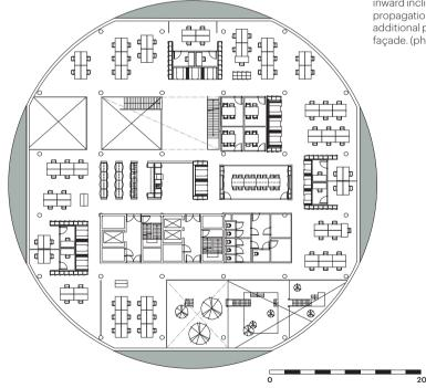
The building's floors have a circular shape. This leads to a favourable ratio between floor space and façade surface, which helps to reduce heat loss. It also leads to shorter walking distances (when compared to a traditional corridor type of floorplan), which allows for easy interaction within the organization.
