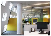
The building has a circular floorplan with an inward inclining façade. This facilitates the propagation of sound. The solve this issue, additional panels have been placed against the façade. (photo: Royal HaskoningDHV)
