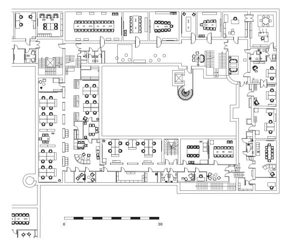
The old building's structure, with its thick walls and narrow floors, lent itself surprisingly well to the ABW concept, allowing the creation of small work areas with 4 to 16 workstations.
