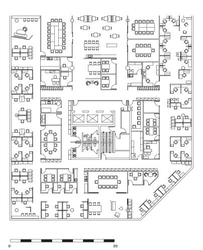
A classic office floor plan with a central core. All the open workstations are located around the floor's perimeter while support spaces, such as small meeting rooms, enclosed offices and storage are located towards the building's core.
